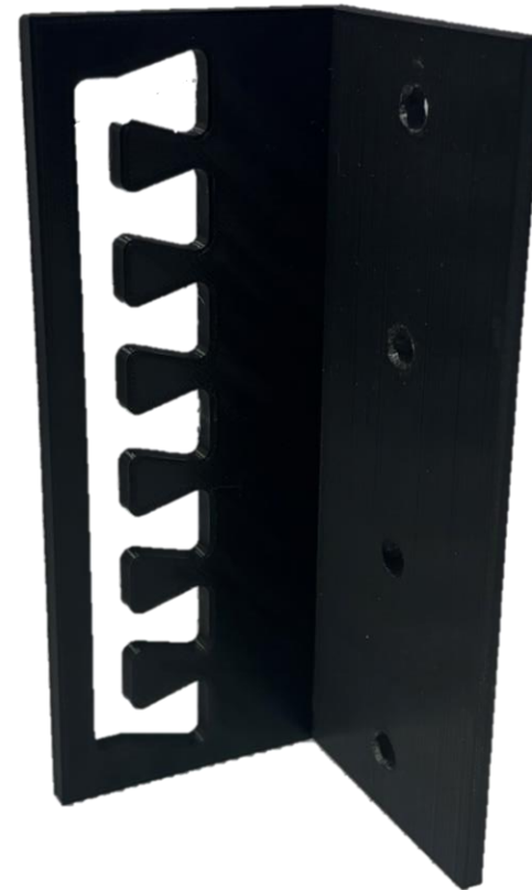
Redesigned Slots for Strength
